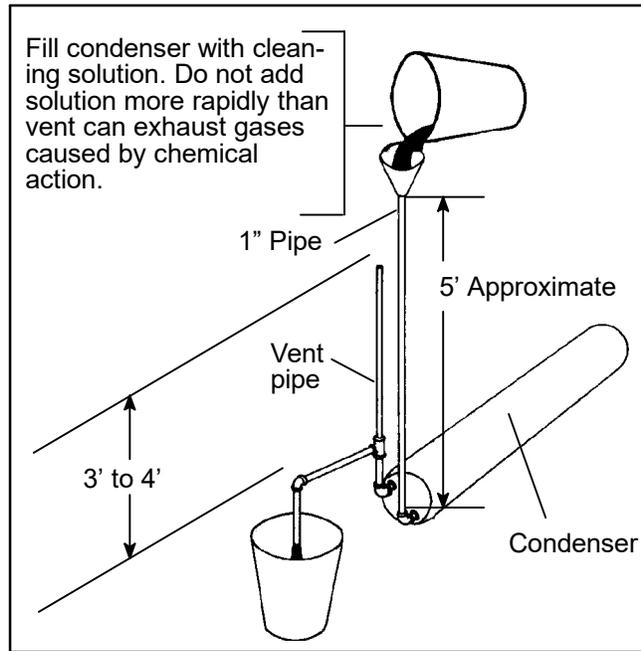
**Figure 39. Water Cooled Condenser Cleaning - Gravity Circulation**
