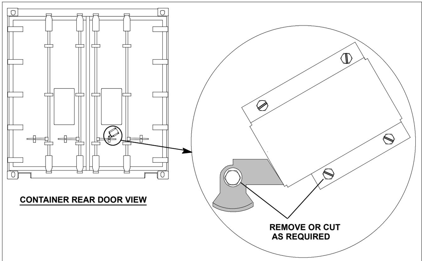
**Figure A. Emergency Bypass for the Door Interlock System**
