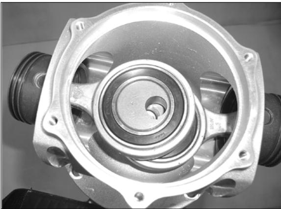
**Figure 75 Rod Assembly Positioning**
