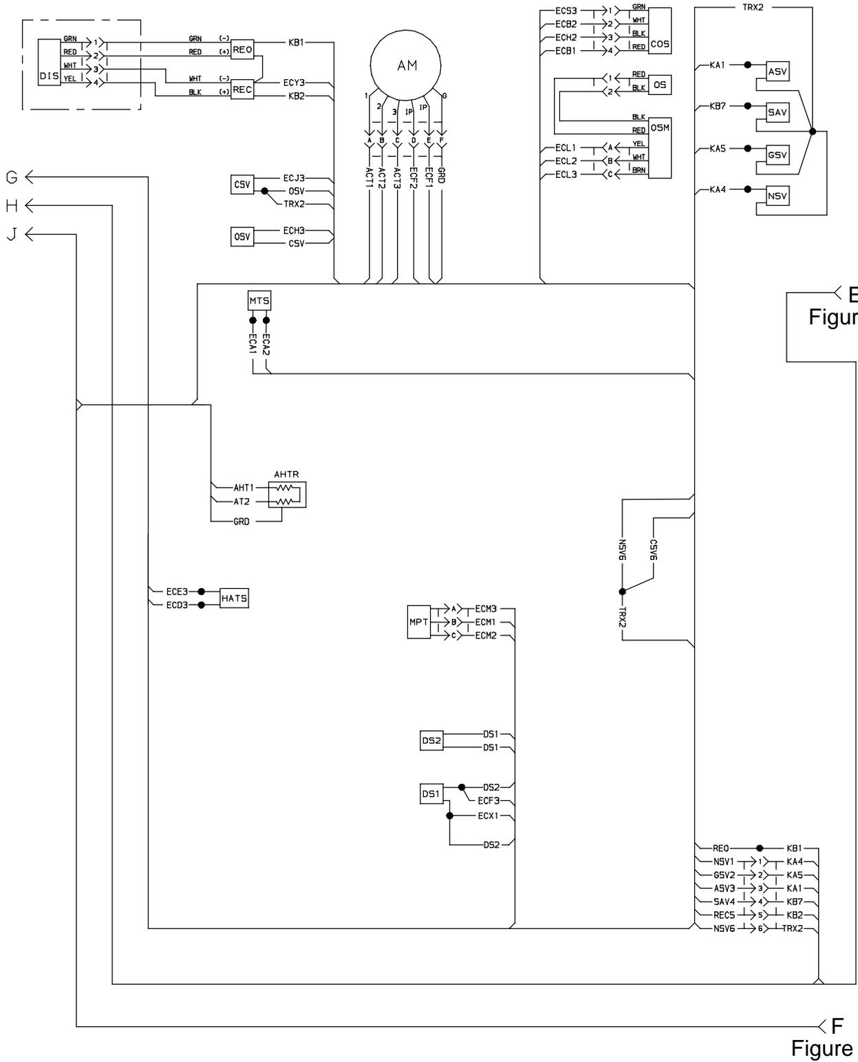
Figure 93. Electrical Wiring Diagram (Sheet 1 of 2)
