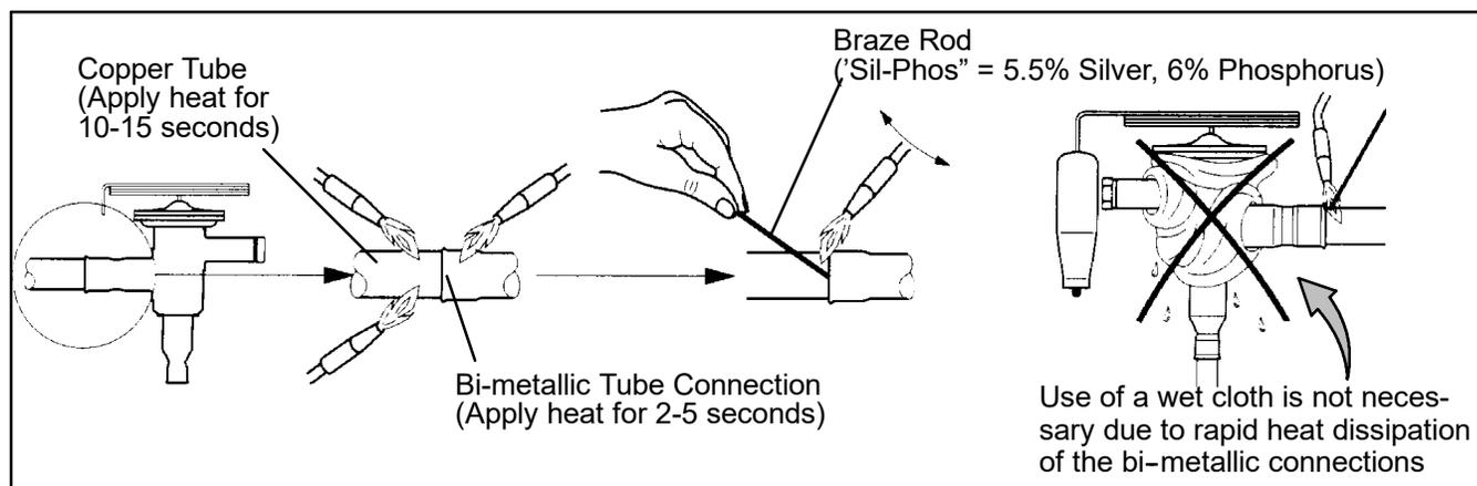
**Figure 42. Hermetic Thermostatic Expansion Valve Brazing Procedure**
