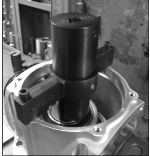
**Figure 76 Rod Pusher Installation**
