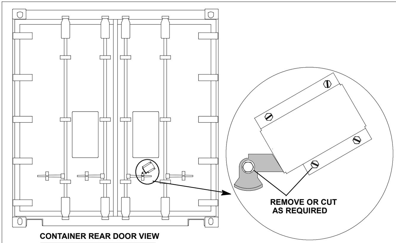
**Figure 66 Emergency Bypass for the Door Interlock System**
