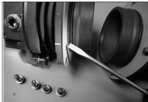
Figure 71 O-Ring Installation
