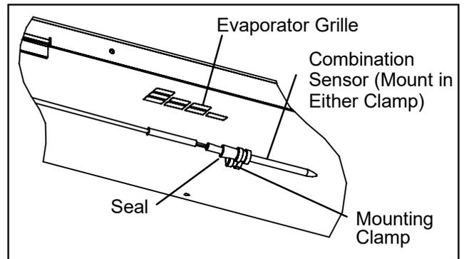
Figure 50. Return Sensor Positioning
