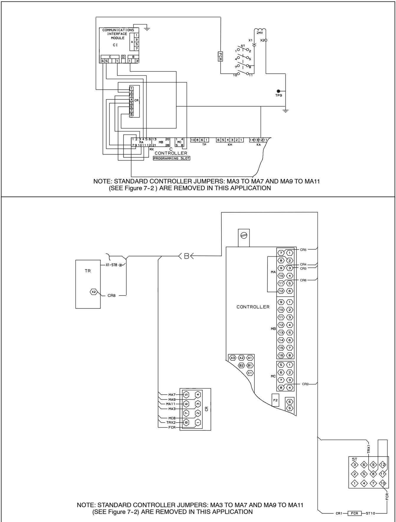
Figure 7-3 SCHEMATIC DIAGRAM, WIRING DIAGRAM- Electronic Partlow Recorder
