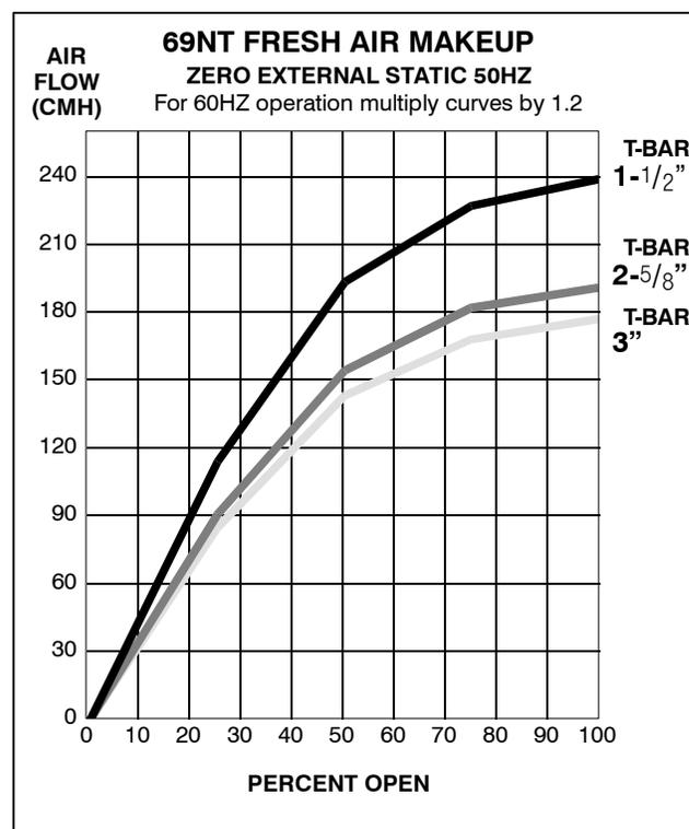
Figure 4-1 Make Up Air Flow Chart
