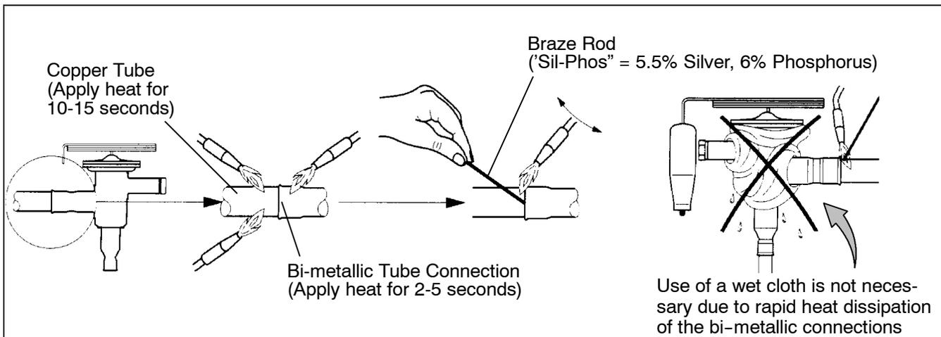
**Figure 6-13 Hermetic Thermostatic Expansion Valve Brazing Procedure**
