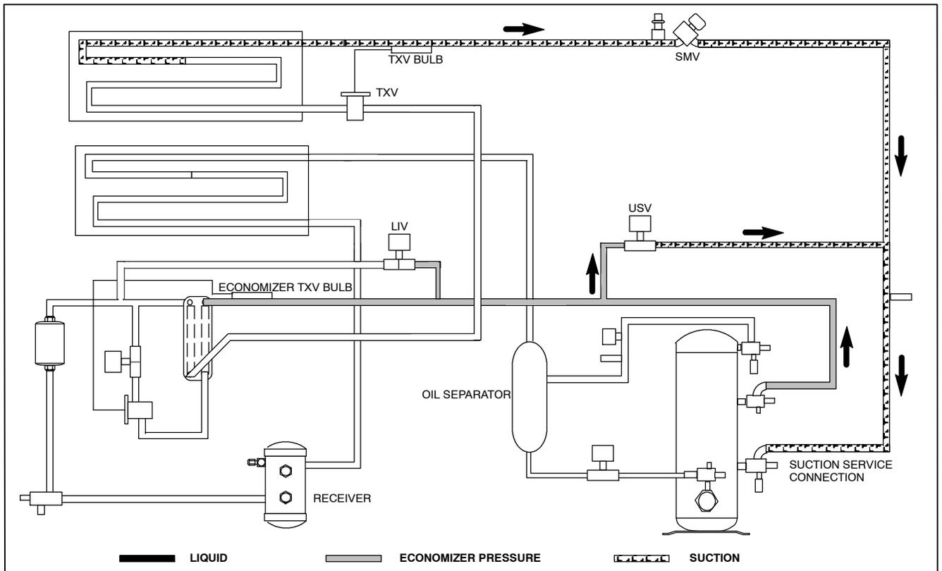
**Figure 2-8 Refrigeration Circuit Schematic - Unloaded Operation**
