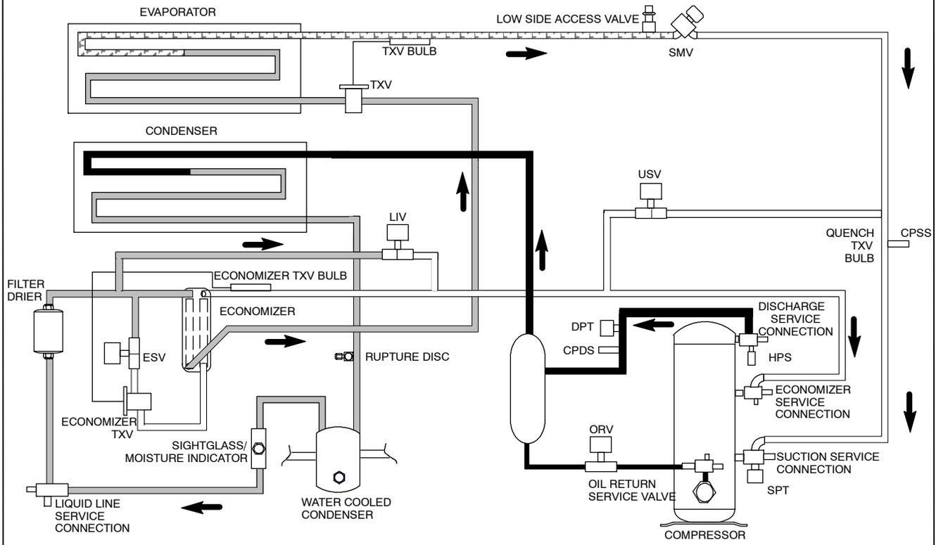
Figure 2-6 Refrigeration Circuit Schematic - Standard Operation
