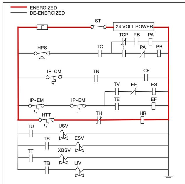
**NOTE:** High-speed, normal operation, single phase evaporator fan shown. For three phase motor units, the compressor is independently operated by an additional (CH) relay. For full diagrams and legend, see Section 7.
