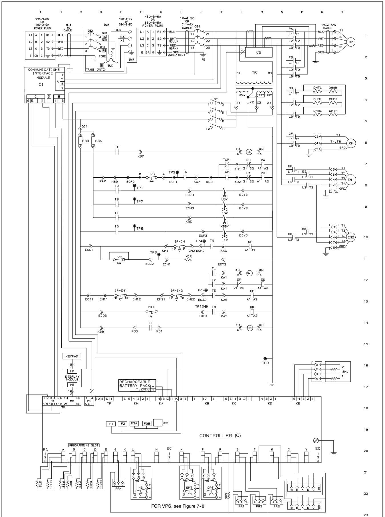
Figure 7-2 SCHEMATIC DIAGRAM - Single Phase, Normal Evaporator Fan Capability
