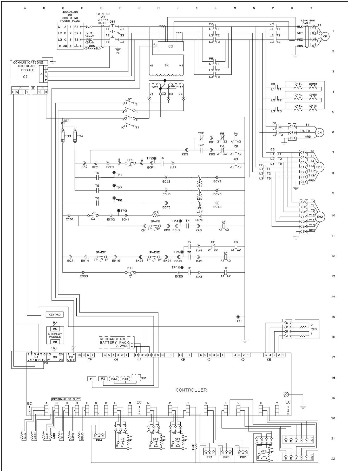
Figure 7-5 SCHEMATIC DIAGRAM - Three-Phase Evaporator Fan Motor
