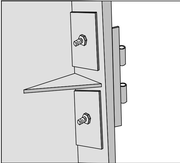
**Figure 6-25 Door Hinge Repair**
