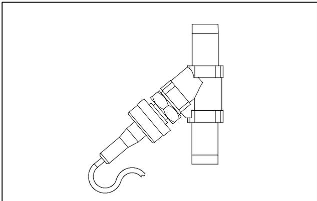
Figure 6-18 Suction Modulation Valve (SMV)
