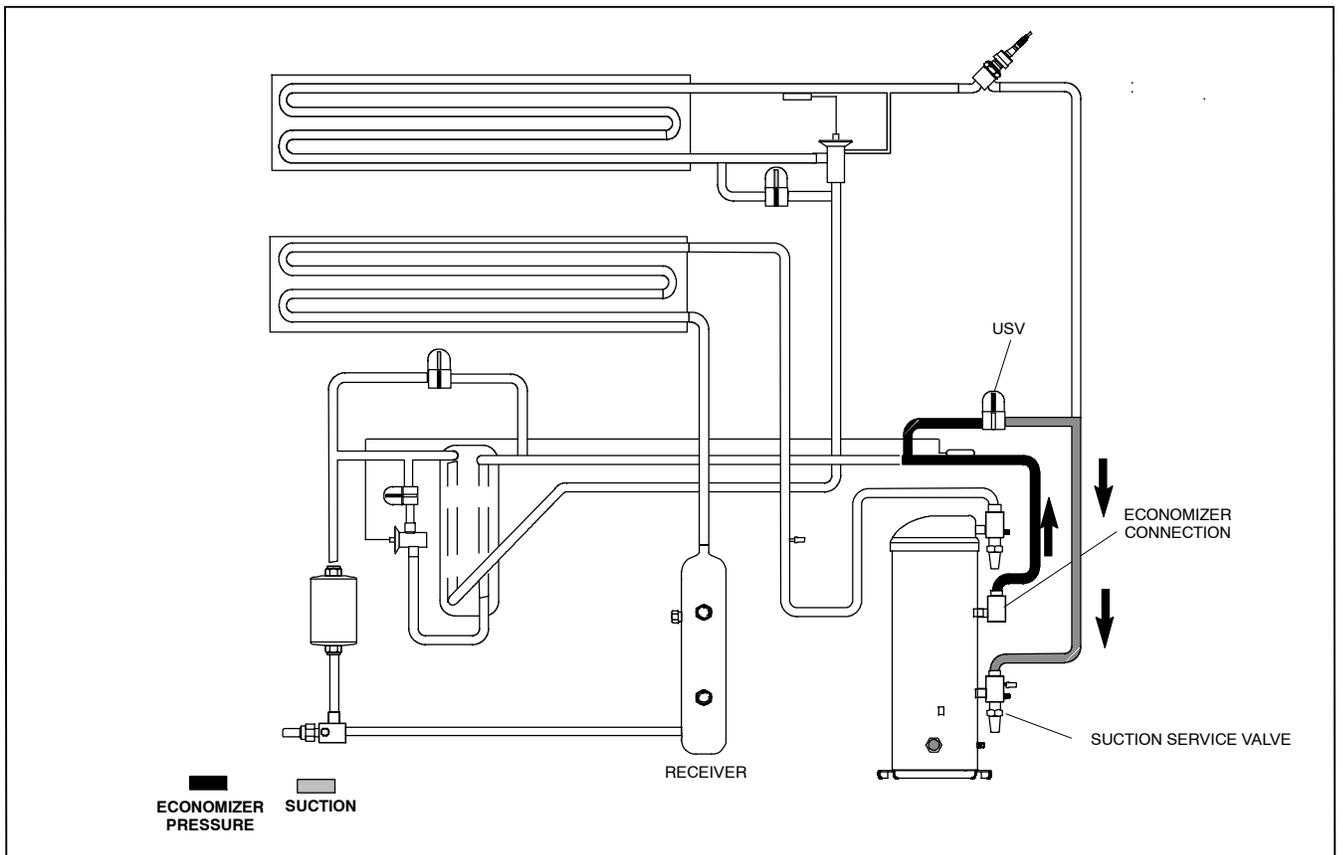
**Figure 2-9 Refrigeration Circuit Schematic - Unloaded Operation**
