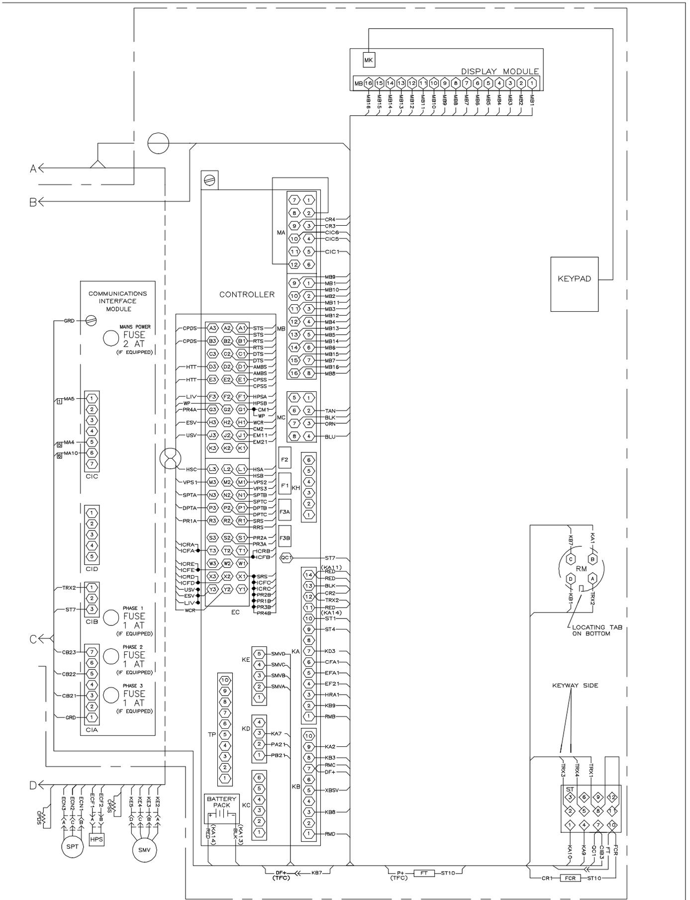
Figure 7-9 WIRING DIAGRAM - Single Phase, Normal Evaporator Fan Capability (Sheet 2 of 2)
