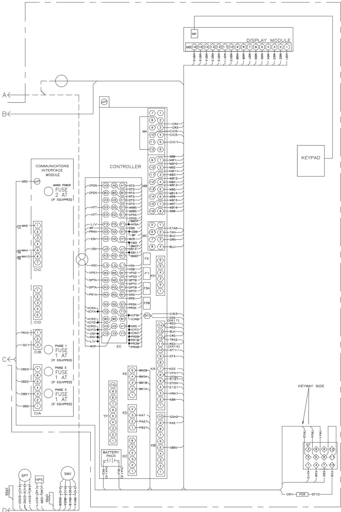
Figure 7-11 WIRING DIAGRAM - Single Phase, Single Evaporator Fan Capability (Sheet 2 of 2)
