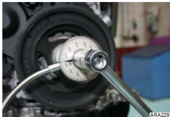
Figure 118: Tighten Bolt 190 Degrees
