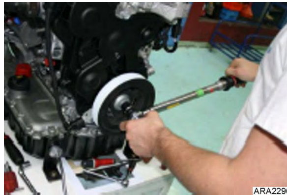
Figure 117: Torque to 25.8 ft-lb (35 N•m)
