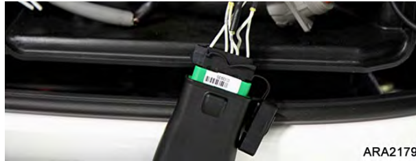
Figure 55: Connect EXXODiag Diagnostic Tool Interface Module to EXXODiag Connector
