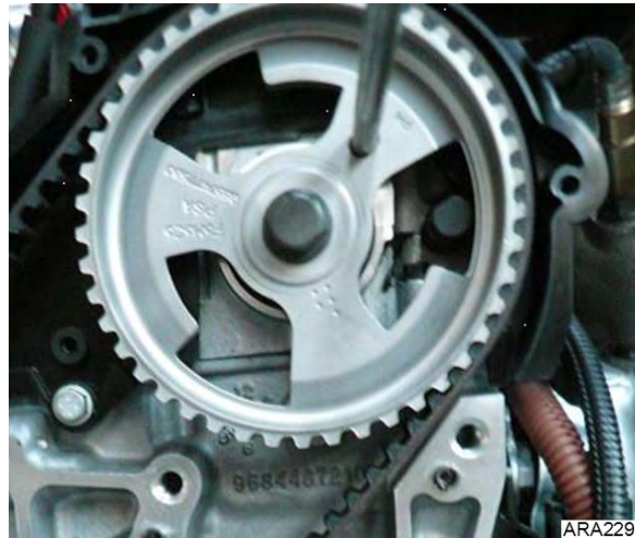
Figure 112: Use 8 mm Locator Pin from Timing Belt Tool Kit P/N 204-2979 to Check Camshaft Pulley Position
