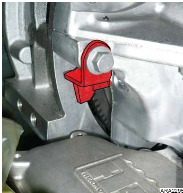
Figure 116: Reinstall Flywheel Locking Tool
