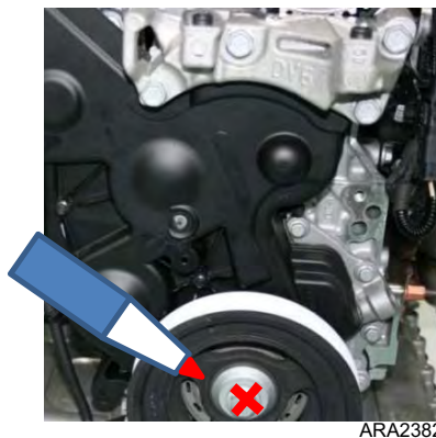
Figure 83: Mark Old Crankshaft Bolt
