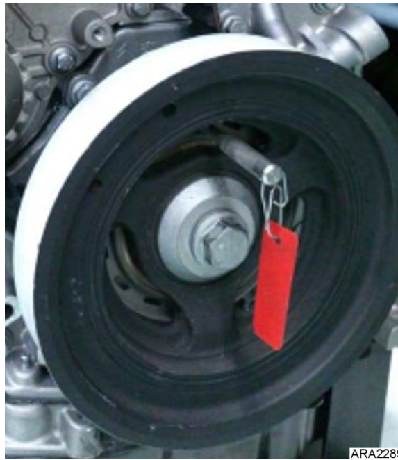
Figure 110: Peg Crankshaft with 5 mm Locator Pin from Timing Belt Tool Kit P/N 204-2979
