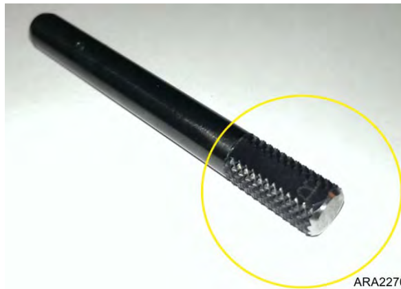
Figure 87: Trim Knurled End if Necessary
