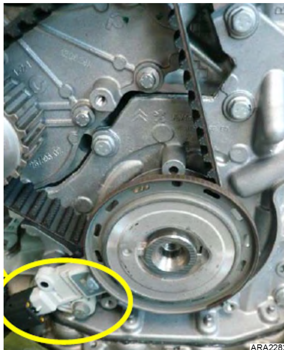
Figure 103: Install Engine Speed Sensor
