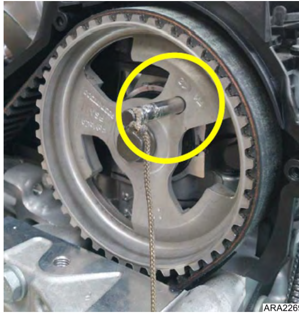
Figure 86: Place Peg in Camshaft and Cylinder Head
