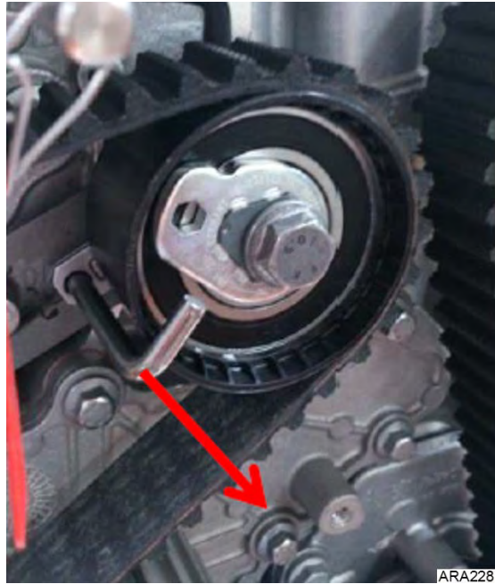
Figure 102: Remove Shipping Key from Belt Tensioner
