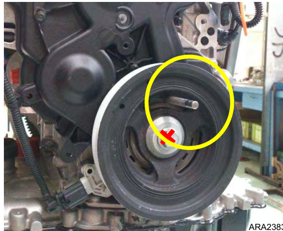
Figure 88: Place Peg in Crankshaft Pulley
