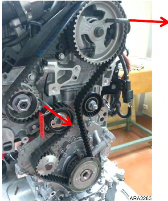
Figure 104: Remove Camshaft and Injection Pump Pin Tools
